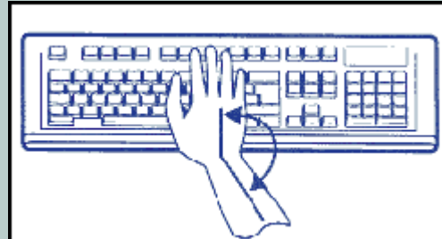
Fig. 1 Hazardous side bending of the wrist.
